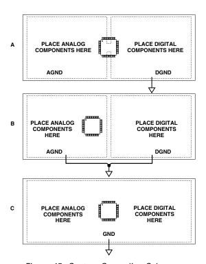
Figure 45. System Grounding Schemes
